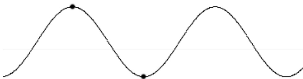
Figure 3.3 To represent a constant sine wave, at least two samples are required for each cycle.
