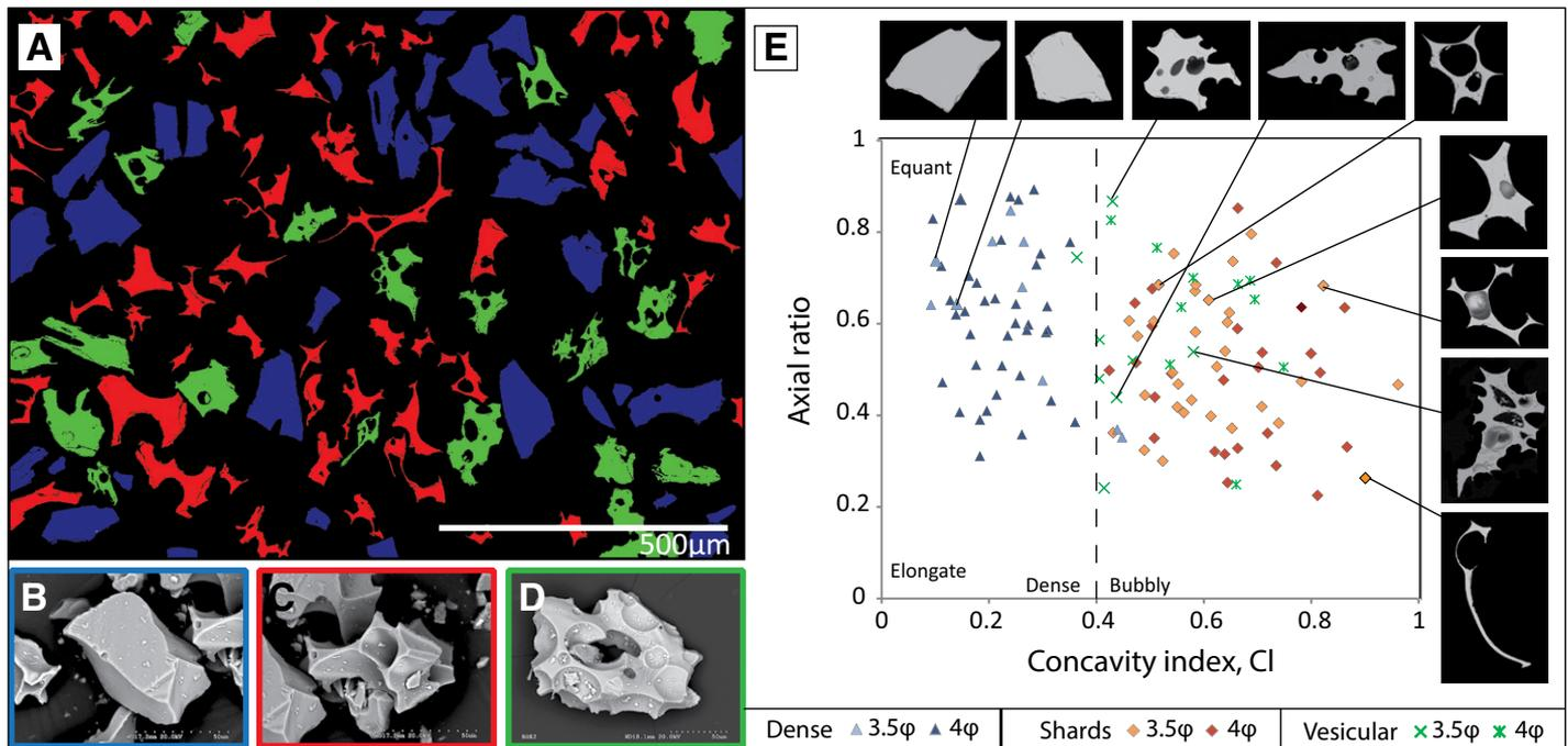
**Figure 2.** Ash characterization by shape analysis. **A:** Backscattered electron (BSE) image from <3.5φ (>91 μm) fraction of sample G6 with pseudo-color overlay highlighting dense fragments (blue), shards (red), and vesicular particles (green). **B–D:** Secondary electron (SE) images of the three components. **E:** Concavity index (CI) versus axial ratio, for components in B–D; dashed line at CI = 0.4 marks threshold between dense fragments and bubbly grains used for automated componentry.
