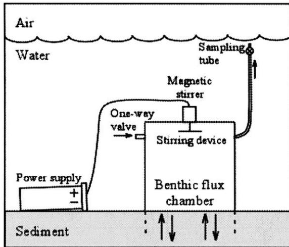
Figure 2. Benthic flux chamber and applied equipment used for direct measurement of solute flux across the sediment–water interface in Lake Myvatn.
