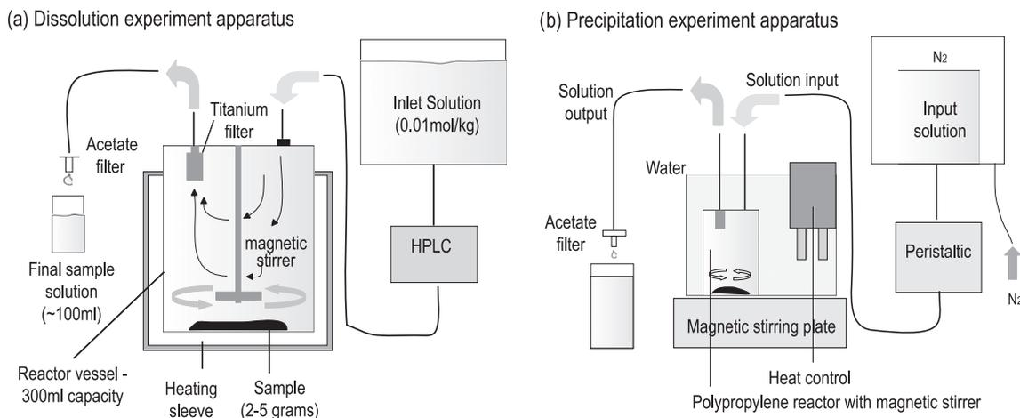
Fig. 1. A schematic diagram showing the experimental apparatus used for (a) dissolution experiments and (b) precipitation experiments.
