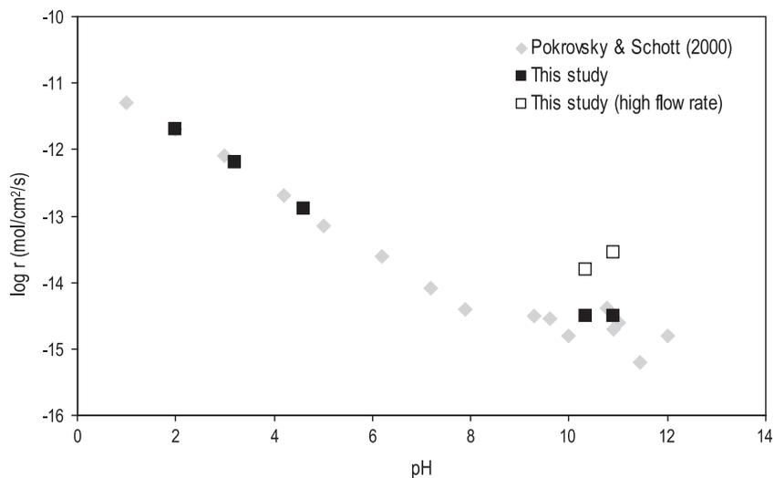
Fig. 10. Comparison of forsterite dissolution rates obtained in this study (at 25 °C, and a constant stir speed) with those published by Pokrovsky and Schott (2000).
