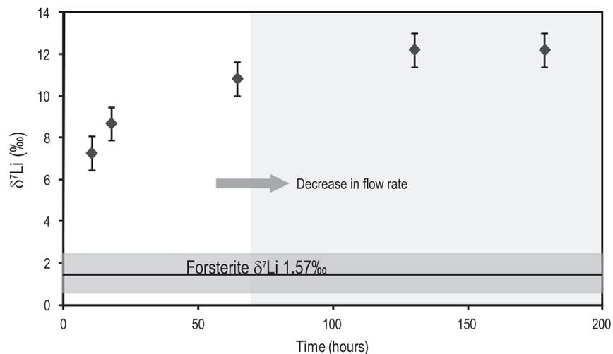
Fig. 6. Lithium isotope ratio of experimental solutions from experiment FO7 (pH 11, 75 °C). Error bars show the external reproducibility ( $2\sigma$ ).
