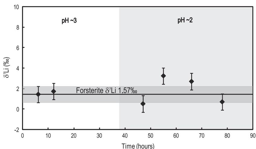
Fig. 2. Lithium isotope ratios of forsterite and experimental fluids during experiment FO2 (pH 2–3, 25 °C). Error bars show the external reproducibility ( $2\sigma$ ).
