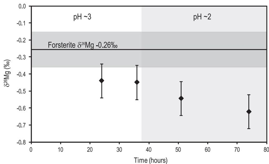
Fig. 3. Magnesium isotope ratio of experimental fluids during experiment FO2 (pH 2–3, 25 °C). Error bars show the external reproducibility (2 $\sigma$ ).
