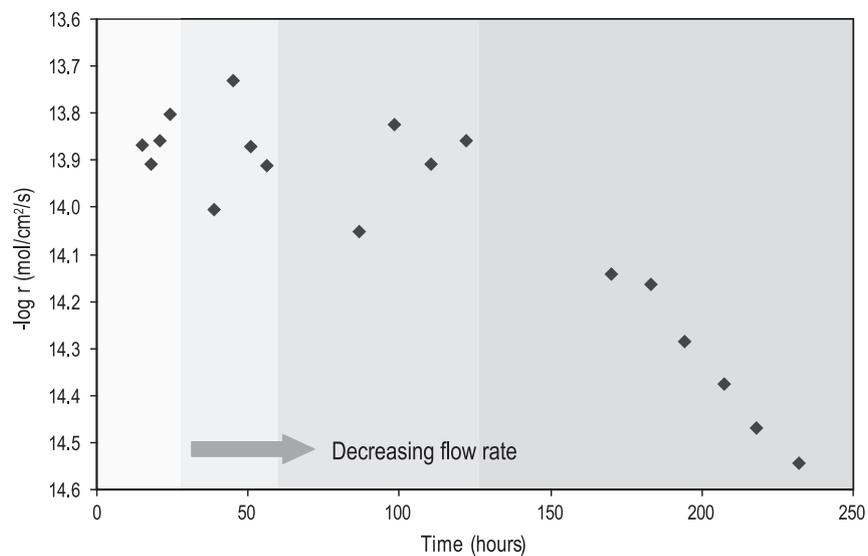
Fig. 4. Dissolution rate of forsterite during the precipitation experiment FO3 (pH 10, 25 °C).
