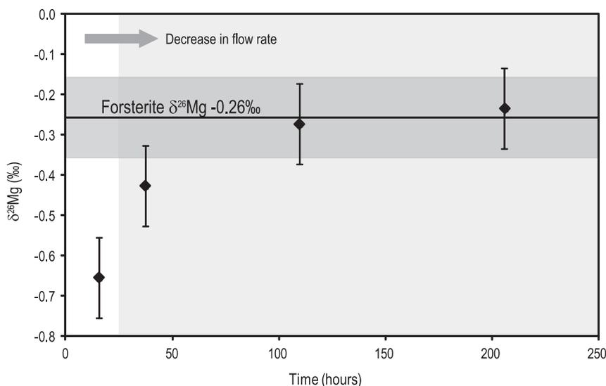
Fig. 7. Magnesium isotope composition of the experimental fluid during dissolution/precipitation experiment FO5 at pH 11 and 25 °C. Error bars show the external reproducibility ( $2\sigma$ ).
