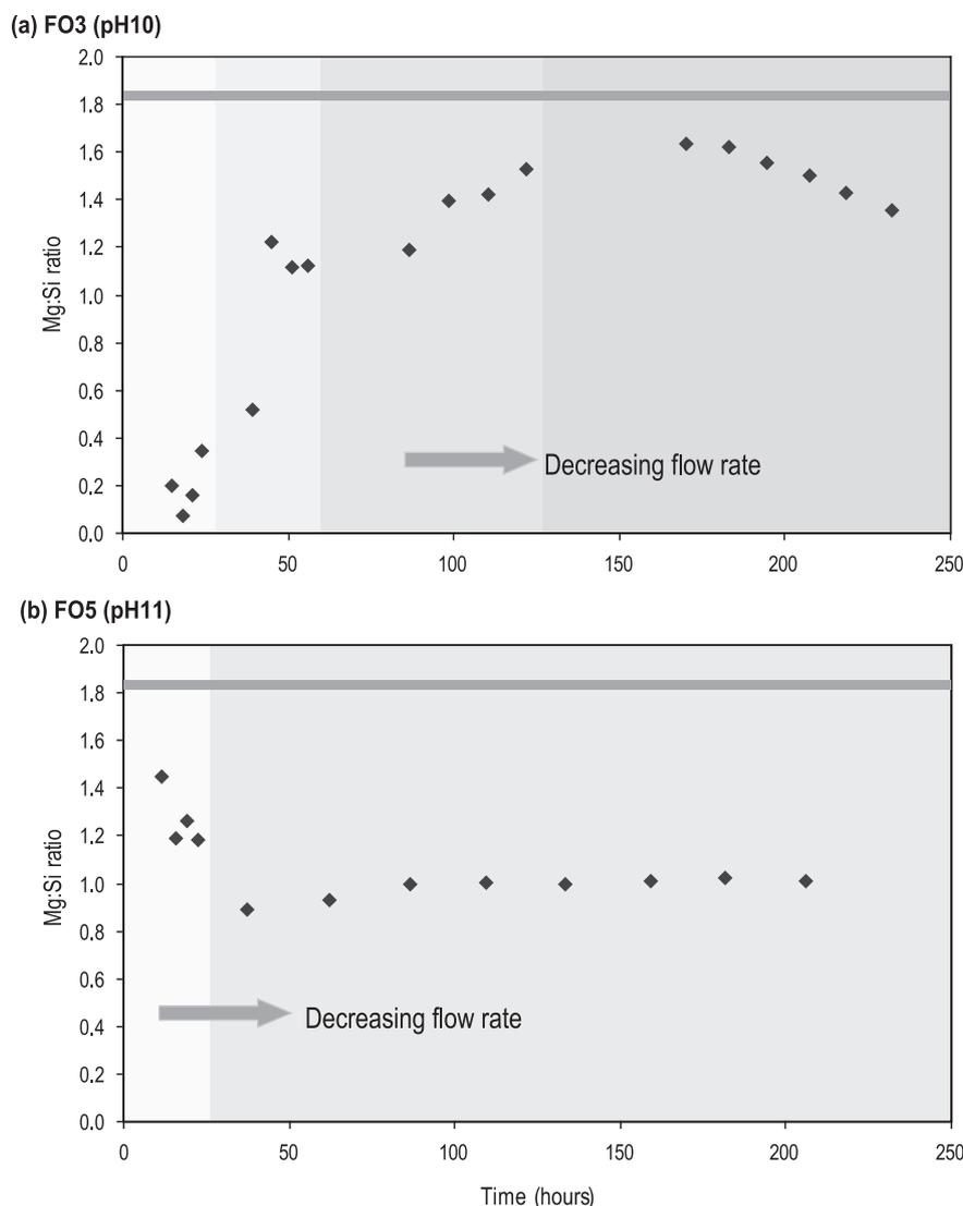
Fig. 8. Mg:Si ratios of experimental solutions from (a) experiment FO3 at pH 10, and 25 °C and (b) experiment FO5 at pH 11. Both experiments were conducted at 25 °C.
