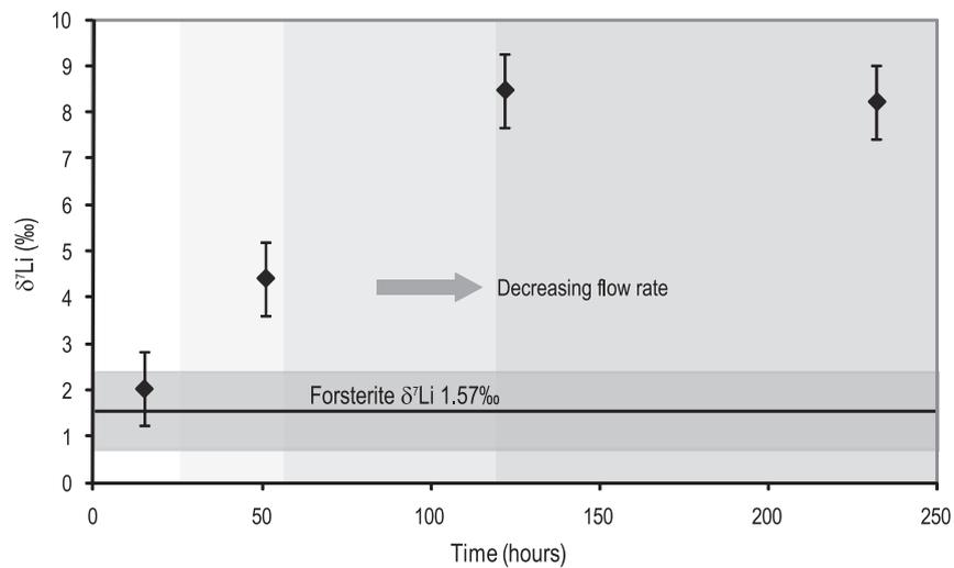
Fig. 5. Lithium isotope composition of experimental fluid during precipitation experiment FO3 (pH 10, 25 °C). Error bars show the external reproducibility ( $2\sigma$ ).
