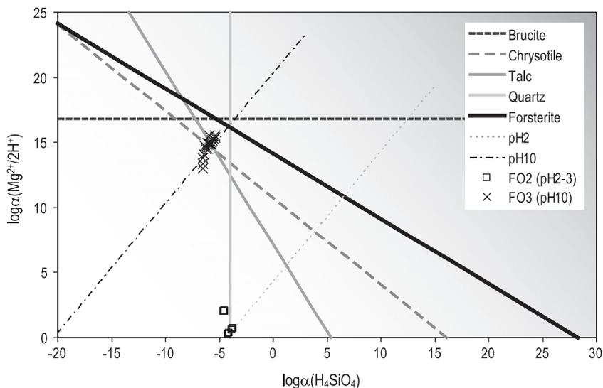
Fig. 9. A magnesium silicate stability diagram showing the saturation state of experimental solutions from experiment FO2 (pH 2–3, 25 °C) and experiment FO3 (pH 10, 25 °C). At pH 2 the experimental solutions are far from equilibrium with respect to Mg-silicates. In contrast at pH 10 the experimental solutions are oversaturated with respect to chrysotile and talc. The equilibrium constants are from the Wateq4f database (Ball and Nordstrom, 1991).
