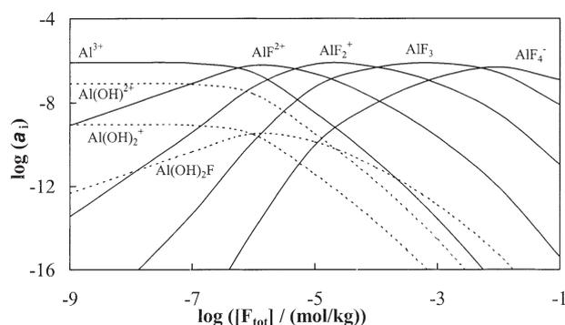
Fig. 1. Computed activities of aqueous  $\text{Al}^{3+}$ ,  $\text{AlF}^{2+}$ ,  $\text{AlF}_2^+$ ,  $\text{AlF}_3^0$ ,  $\text{AlF}_4^-$ ,  $\text{Al}(\text{OH})^{2+}$ ,  $\text{Al}(\text{OH})_2^+$ , and  $\text{Al}(\text{OH})_2\text{F}^0$  as a function of the total aqueous F concentration at pH 4 and 25°C. The curves were generated with PHREEQC 2.6 and for a solution having a total aluminium concentration of  $10^{-6}$  mol/kg.
