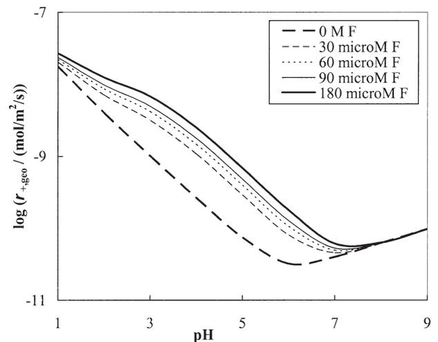
Fig. 9. The logarithm of  $r_{+geo}$  versus the pH for the rhyolitic glass BT. The curves were all calculated using Eqn. 8. The aqueous activities were computed with PRHEEQC 2.6 at a total Al concentration of  $10^{-6}$  mol/kg and the fluoride concentrations given in the legend. The bold dashed line represents  $r_{+geo}$  as a function of pH in the absence of aqueous fluoride. The other four lines display how  $r_{+geo}$  increases with increasing F concentration.
