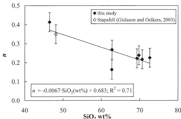
Fig. 5. The stoichiometric coefficient  $n$  (Eqn. 1 and 2) as a function of the silica content of the glasses. The symbols correspond to  $n$  values generated from the slopes of the fits illustrated in Figure 4. The line through the data represents a linear least square fit of  $n$  from the values of this study; the equation and correlation coefficient ( $R^2$ ) of this fit are provided. The error bars correspond to an estimated  $\pm 0.05$  uncertainty in  $n$ .
