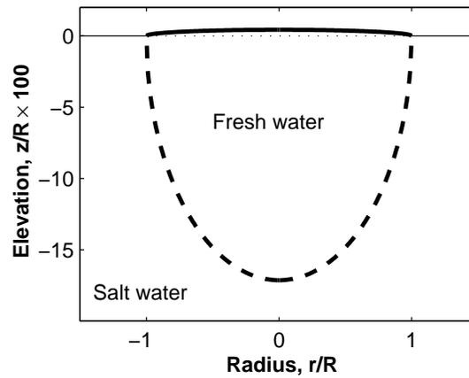
Figure 10.10 shows a sketch of the situation on an island with a pumping well where the pumping rate exceeds the natural recharge. If pumping continues at this rate, the well may start pumping up sea water in the near future.
