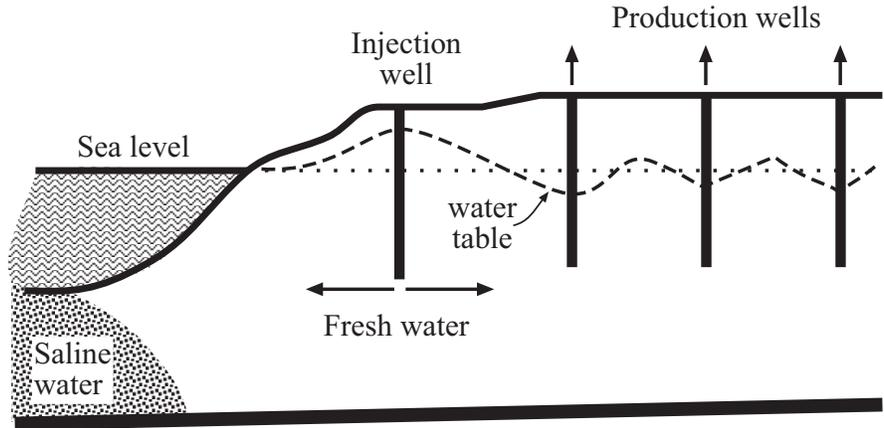
**Fig. 10.7** Artificial recharging is used to raise the water table closest to the shore such that the fresh water flow is towards the shore.
