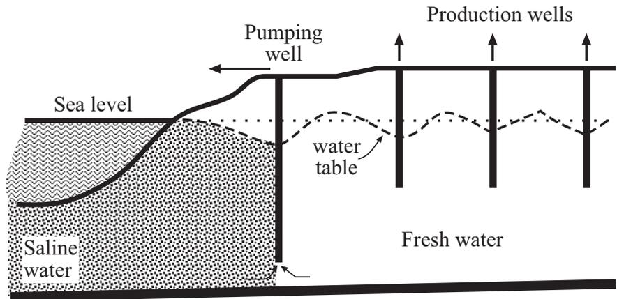
**Fig. 10.8** Many well are lined up in parallel along the coastline, generating a drawdown that will limit the intrusion of sea water.
