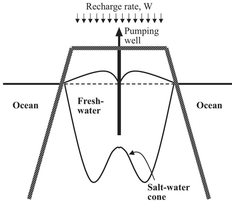
**Fig. 10.10** Sketch of an oceanic island with a pumping well.
