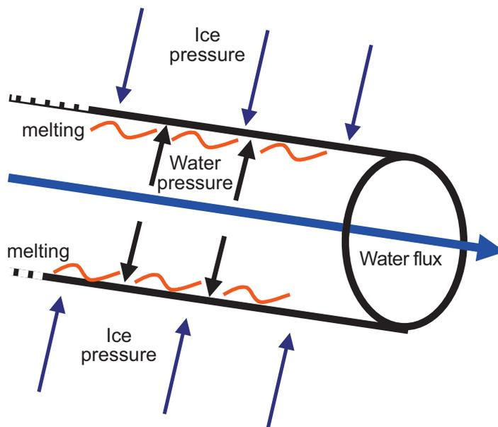
**Fig. 8.5** Schematic of a tunnel. There is competition between melting (and water pressure) expanding the tunnel, and ice deformation trying to close it.
