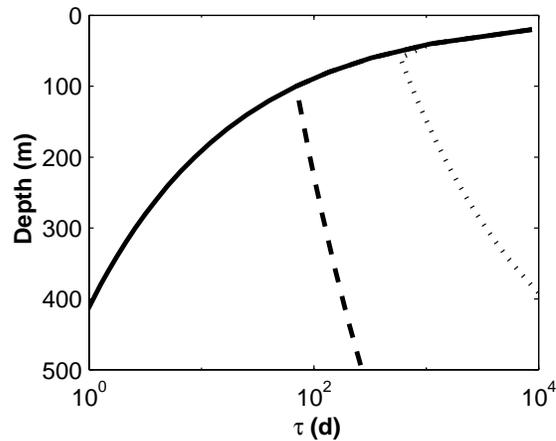
**Fig. 8.6** The time-scale for closure assuming that there is no water in the bore-hole (solid line), that the water table is 50 m (dotted line) and 100 m (dashed line) below the ice surface.
