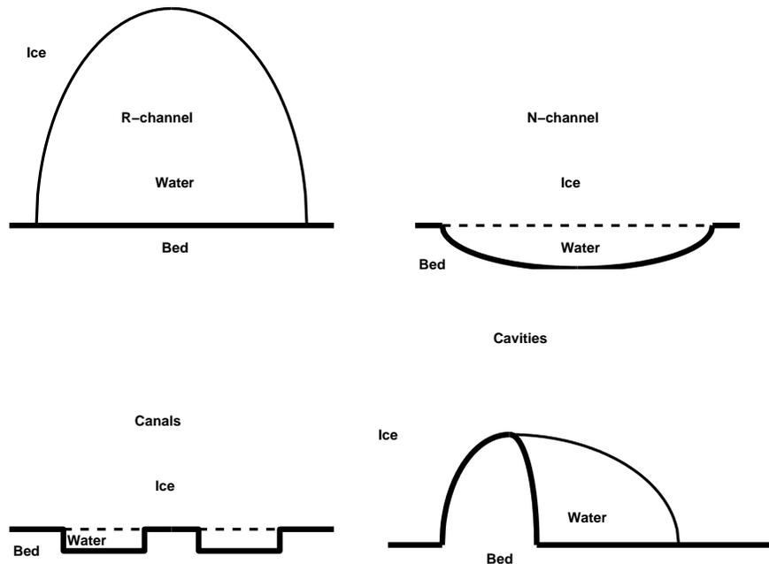
**Fig. 8.9** Schematic of tunnels and channels at the bed. Röthlisberger-channels are cut up into the ice, Nye-channels are cut into the bedrock, canals are shallow and broad features in sediments, and cavities form on the lee side of bedrock bumps.
