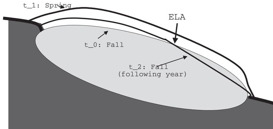
**Fig. 7.1** Equilibrium Line Altitude (ELA). The surface at fall  $t_0$ , after the winter accumulation in spring  $t_1$  and the following fall  $t_2$ .
