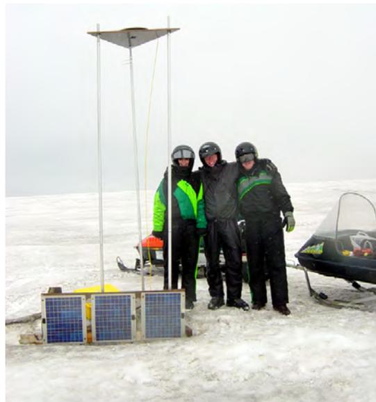
**Fig. 7.4** Ablation at Mýrdalsjökull, S-Iceland. The triangular platform was 20 cm above the surface in late April. When this picture was taken, in late June, it stood 3 m above the surface. Picture Throstur Thorsteinsson, 2003.
