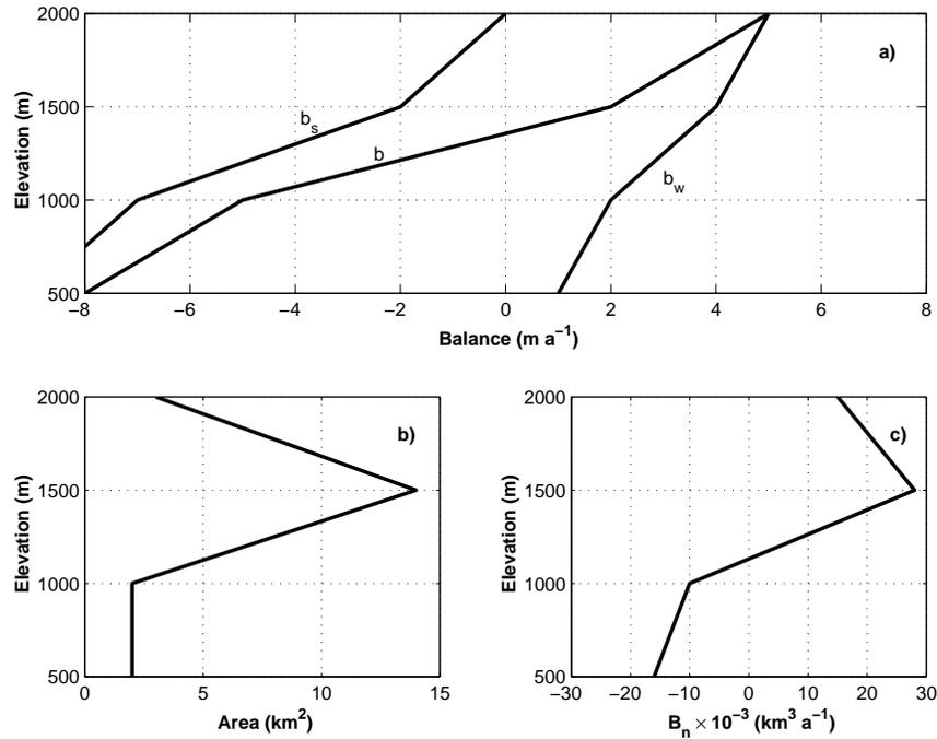
**Fig. 7.3** Mass balance data. a) Plot of summer- ( $b_s$ ), winter- ( $b_w$ ) and net-balance ( $b$ ) with height, b) area distribution with height, and c) area weighted balance  $B_n$ .
