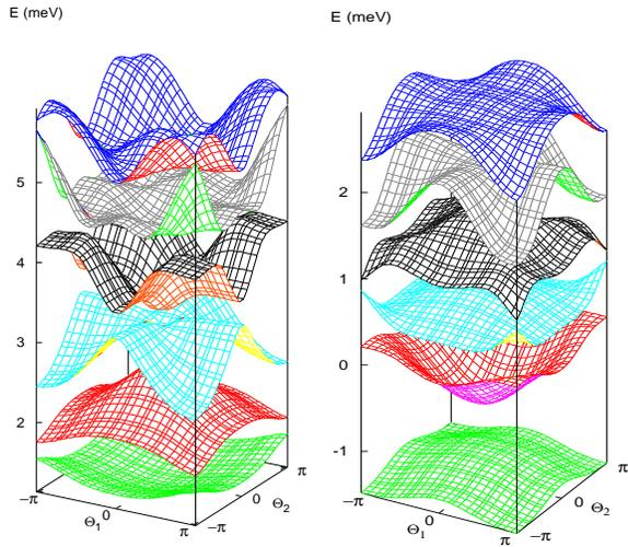
FIG. 1. The energy spectra in the first Brillouin zone for quantum antidots (left), and dots (right).  $pq = 1$ ,  $V = \pm 5$  meV,  $N_s = 0.5$ ,  $L = 100$  nm, and  $T = 1$  K.
