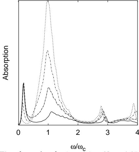
FIG. 4. The absorption for increasing  $N_s = 0.25$  (solid), 0.50 (dashed), 0.75 (dashed-dotted), and 1.00 (dots) in the case of  $\mathbf{k}L = (0.2, 0)$ ,  $pq = 1$ ,  $V = 5$  meV,  $L = 100$  nm, and  $T = 1$  K.
