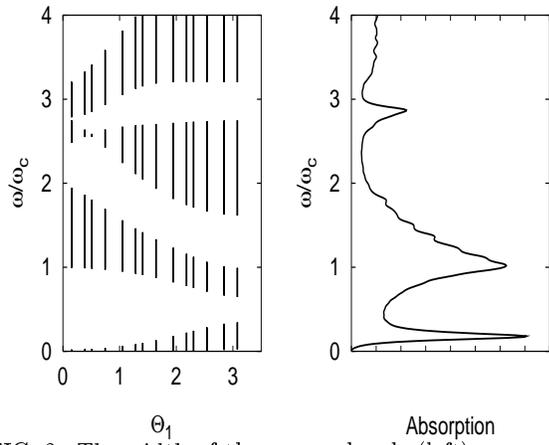
FIG. 3. The width of the energy bands (left) compared to the absorption (right) in the case of  $\mathbf{k}L = (0.2, 0)$ ,  $pq = 1$ ,  $N_s = 0.5$ ,  $V = 5$  meV,  $L = 100$  nm, and  $T = 1$  K. The zero of the energy bands coincides with the chemical potential  $\mu$ .
