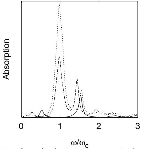
FIG. 5. The absorption for increasing  $N_s = 0.5$  (solid), 2.0 (dashed), 3.0 (dots) in the case of  $\mathbf{k}L = (0.2, 0)$ ,  $pq = 3$ ,  $V = -5$  meV,  $L = 100$  nm, and  $T = 1$  K.
