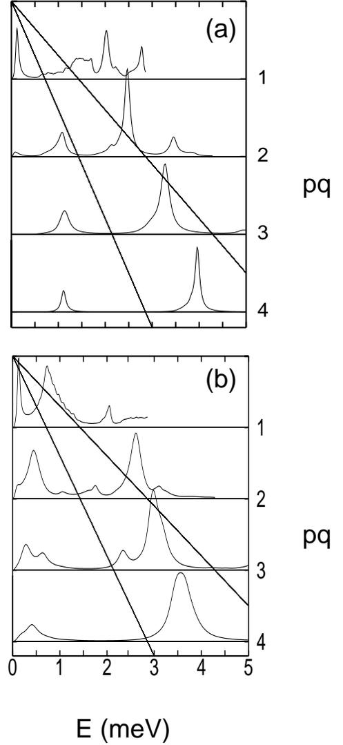
FIG. 2. The Power absorption as a function of  $E = \hbar\omega$  and the number magnetic flux units  $pq$  in a unit cell for dots (a), and antidots (b).  $\mathbf{k}L = (0.2, 0)$ ,  $N_s = 0.5$ ,  $V = \pm 5$  meV,  $L = 100$  nm, and  $T = 1$  K. The damping parameter is  $\hbar\eta = 0.05\hbar\omega_c$  except in (a) for  $pq = 4$  it is half this value. The straight lines representing  $E = \hbar\omega_c$ , and  $E = 2\hbar\omega_c$  are shown as a guide to the eye.
