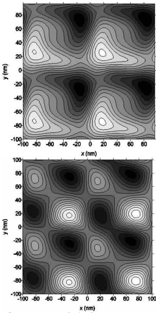
FIG. 7. The induced density for quantum antidots for  $E = 0.63$  meV,  $kL = (0.2, 0)$ ,  $pq = 3$  (upper panel), and  $E = 1.74$  meV,  $pq = 2$  (lower panel).  $N_s = 0.5$ ,  $V = 5$  meV,  $L = 100$  nm, and  $T = 1$  K.
