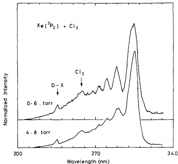
Fig. 2. XeCl  $B \rightarrow X$  emission spectra from the reaction of  $\text{Xe}(^3P_2)$  metastables with  $\text{Cl}_2$  in a flowing afterglow with Ar buffer at 0.6 and 4.8 Torr
