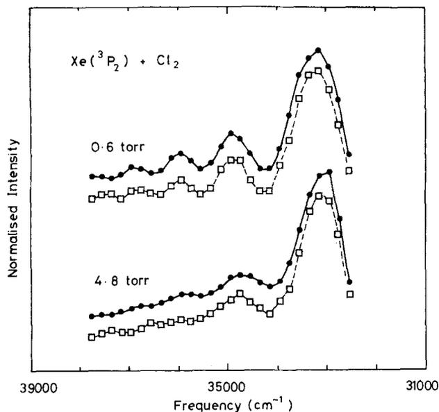
Fig. 4. XeCl  $B \rightarrow X$  spectra. Solid line: as digitised from the experimental spectra shown in Fig. 2. Dotted line: spectra recalculated from the population histograms
