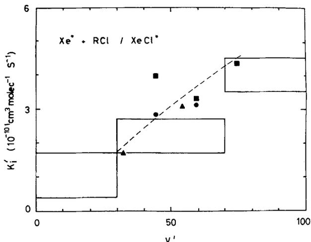
Fig. 6. Effective vibrational relaxation rate constants as a function of vibrational level for XeCl+Ar. Triangles: Xe( $^3P_2$ +CCl $_4$  at 4.8 Torr, circles: Xe( $^3P_1$ )+Cl $_2$  at 10.8 Torr, squares: Xe( $^3P_1$ )+Cl $_2$  at 5.4 Torr. The large open boxes give the limits of the sum of relaxation and inter-system crossing rate constants from [12]
