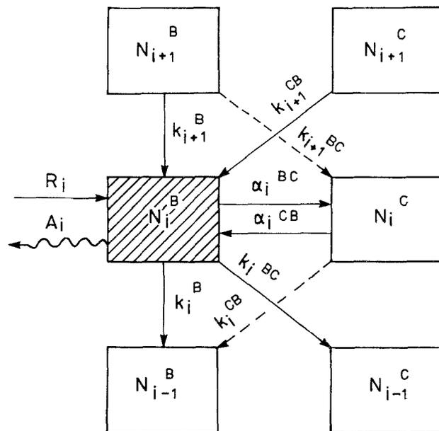
Fig. 5. Gain and loss processes affecting a single block of vibrational levels in the  $B$  state
