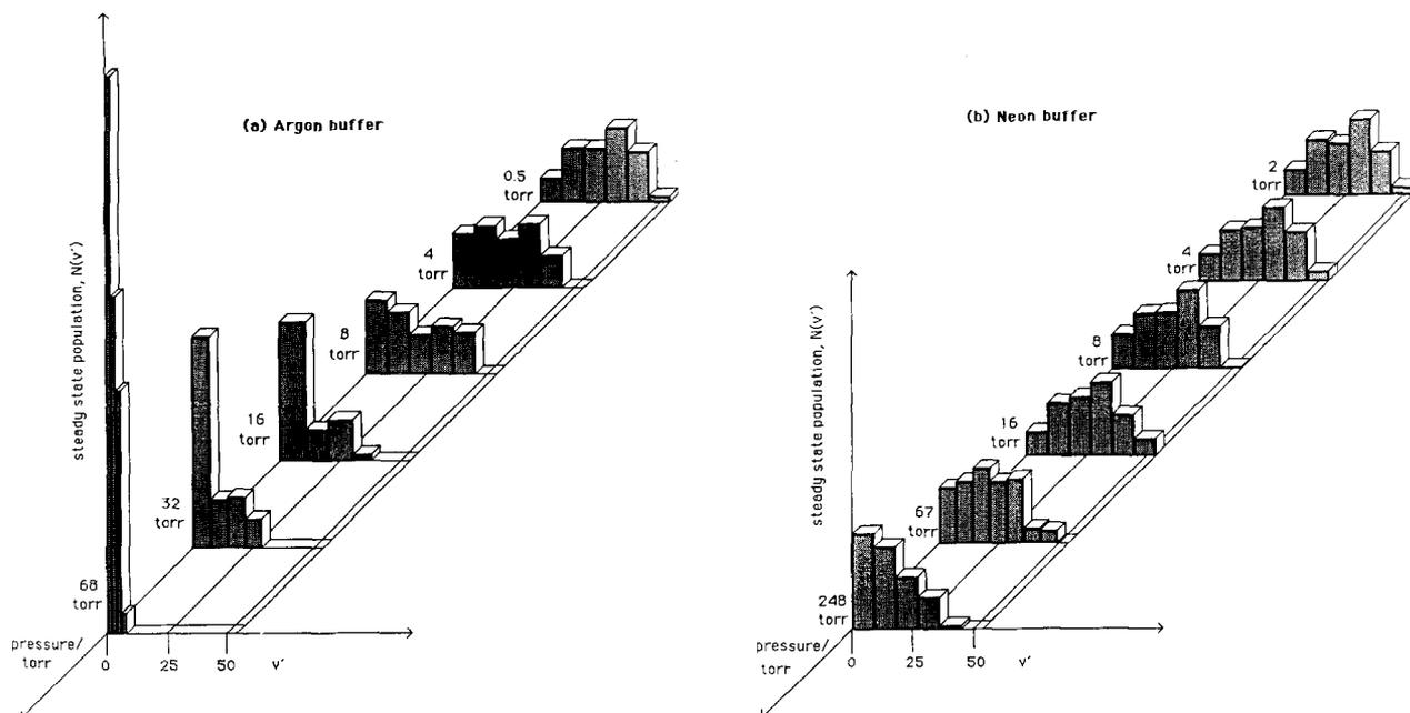
Fig. 3. Histograms of vibrational populations in the KrF  $B$  state corresponding to the spectra of Fig. 1. Histograms are normalised so that the total number of particles in each histogram is constant
