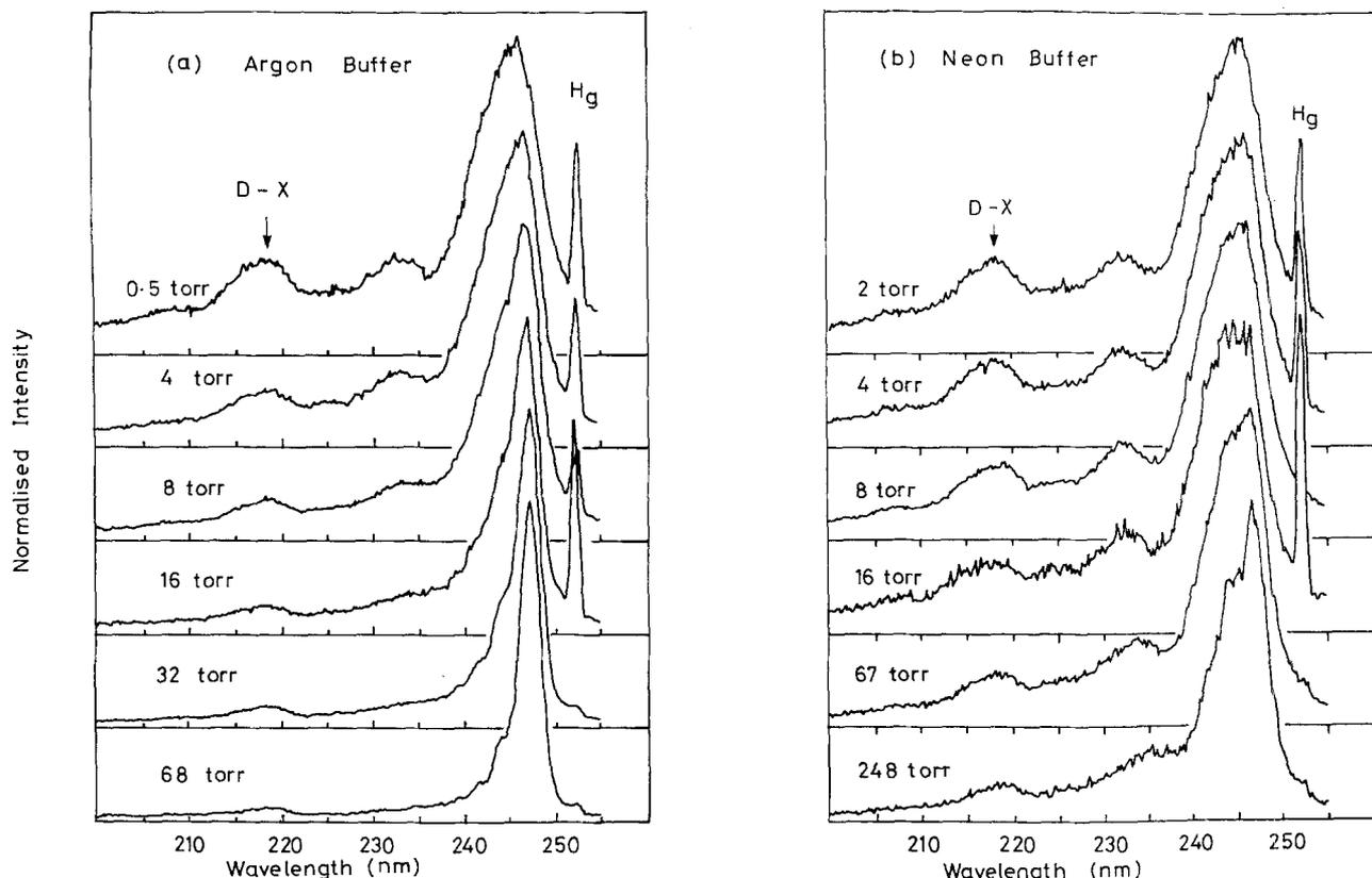
Fig. 1a, b. KrF  $B \rightarrow X$  emission spectra excited by Kr resonance radiation illumination of 0.25 Torr Kr + 0.25 Torr  $\text{NF}_3$  + buffer gas to total pressure shown. (a) Ar buffer; (b) Ne buffer
