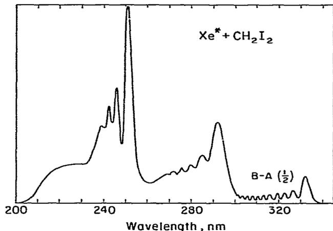
Fig. 4.  $\text{XeI}^*$  spectrum generated by  $\text{Xe}^* + \text{CH}_2\text{I}_2$ . Total pressure: 0.8 torr.
