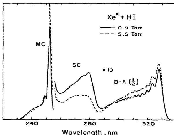
Fig. 3.  $XeI^*$  spectra generated by  $Xe^* + HI$ . Integrated intensities at the two pressures are equal.
