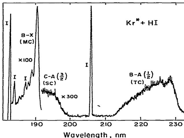
Fig. 2.  $KrI^*$  spectrum generated by  $Kr^* + HI$  at 2.1 torr total pressure. Iodine lines at 184.5, 187.6 and 206.2 nm arise from  $Ar^* + HI$ .
