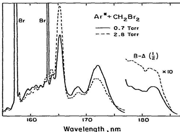
Fig. 5.  $\text{ArBr}^*$  spectra generated by  $\text{Ar}^* + \text{CH}_2\text{Br}_2$ . The integrated intensities at the two pressures are equal.
