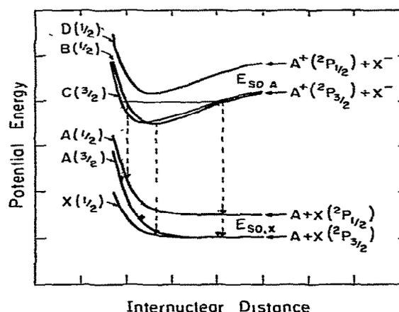
Fig. 1. Schematic potential curves for the noble-gas halides, AX.  $E_{SO,A}$  ( $\text{cm}^{-1}$ ): Ar: 1432; Kr: 5371; Xe: 10537.  $E_{SO,X}$  ( $\text{cm}^{-1}$ ): Br: 3685; I: 7603. --- Transitions from B(1/2), . . . transitions from C(3/2).
