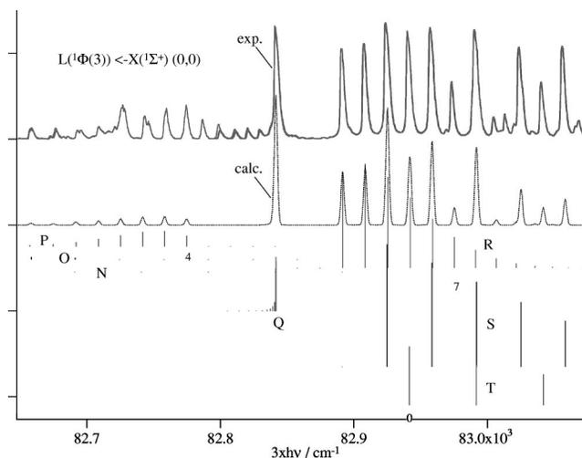
FIG. 4. HBr,  $L(^1\Phi(3)) \leftarrow X(^1\Sigma^+)$ , (0,0) (3+1)REMPI spectrum analysis: Observed (3+1)REMPI spectrum (top), calculated rotational line contributions (bottom) and simulated spectrum (underneath exp. spectrum). Rotational line numbers are  $J''$  values. Some unidentified overlapping spectrum is to be found in the region 82 650–82 830  $\text{cm}^{-1}$ .
