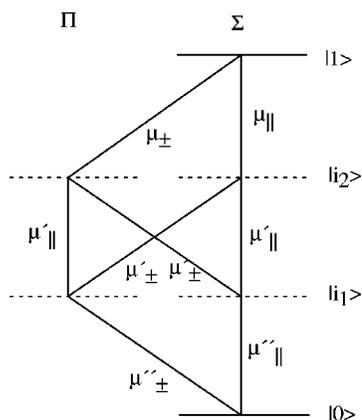
FIG. 1. Structure of the three-photon transition amplitude for a diatomic molecule showing intermediate/virtual states and one-photon transition moments for  $\Sigma \leftarrow \Sigma$  ( $\Omega = 0 \leftarrow \Omega = 0$ ) overall transitions.
