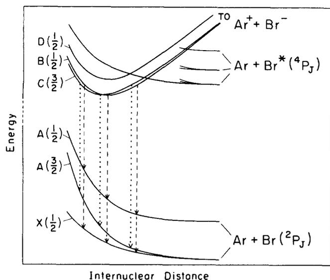
FIG. 4. Schematic potential curves of ArBr, with the transitions observed in this study. See Fig. 5 for the ordering of the Br spin-orbit levels.
