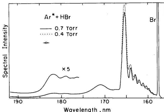
FIG. 1. Chemiluminescence spectrum of the reaction of  $\text{Ar}^*(^3P_{0,2})$  with HBr. The high- and low-pressure spectra are normalized to constant Br-line intensity. Monochromator spectral resolution: 0.2 nm.
