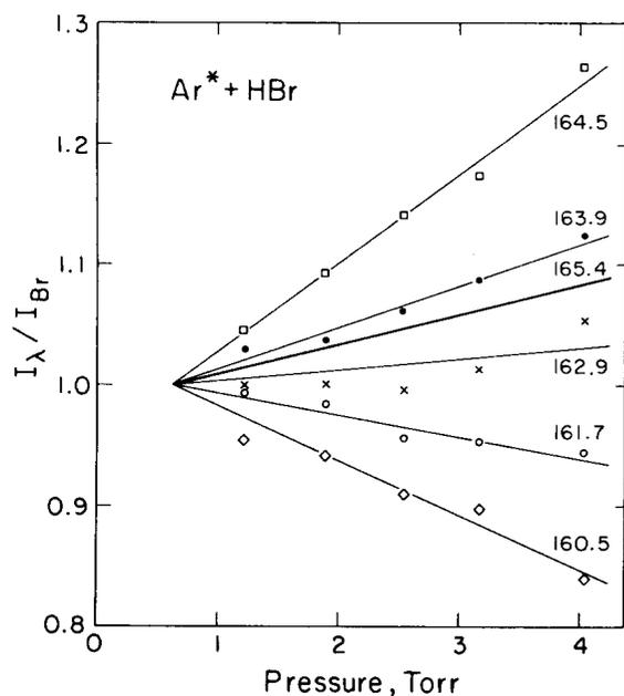
FIG. 6. Pressure dependence of emission intensity at selected wavelengths in the main continuum of  $\text{Ar}^* + \text{HBr}$ . Ordinate: ratio of  $\text{ArBr}$  emission intensity to that of the 157.7 nm Br line. All data normalized to unity at 0.6 Torr.
