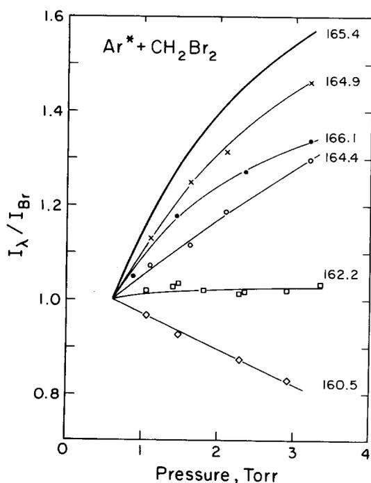
FIG. 7. Pressure dependence of emission intensity at selected wavelengths in the main continuum of  $\text{Ar}^* + \text{CH}_2\text{Br}_2$ . See caption to Fig. 6 for details.
