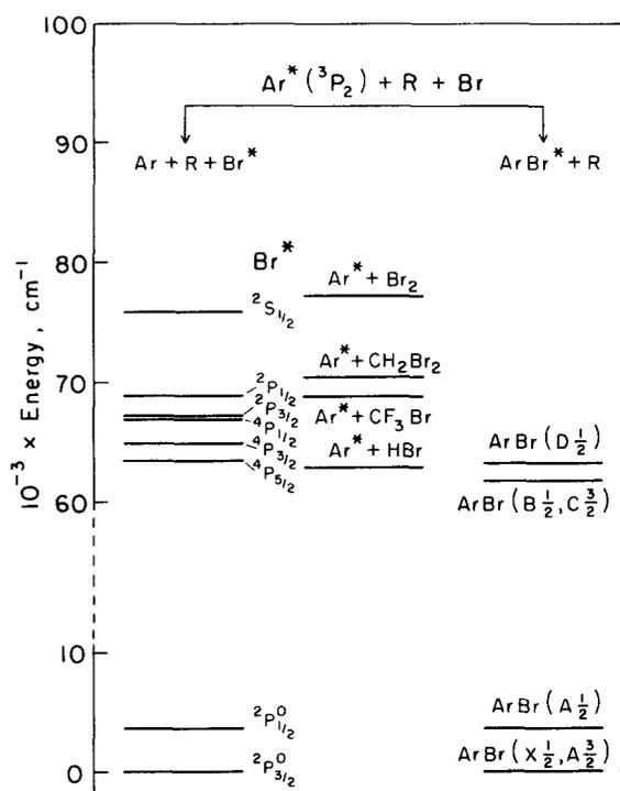
FIG. 5. Energy level diagram, illustrating the electronic states of ArBr and Br accessible in the reactions studied.
