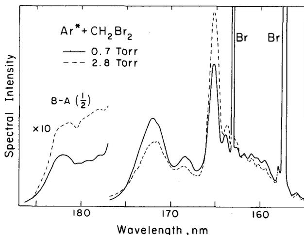
FIG. 2. Chemiluminescence spectrum of the reaction of  $\text{Ar}^*(^3P_{0,2})$  with  $\text{CH}_2\text{Br}_2$ . The high- and low-pressure spectra are normalized to constant atomic Br emission intensity.
