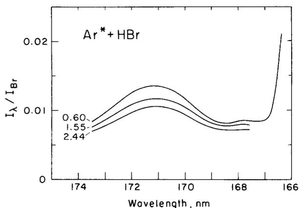
FIG. 8. Pressure dependence of the secondary continuum of  $\text{Ar}^* + \text{HBr}$ . Pressures given in Torr. Ordinate: Absolute ratio of  $\text{ArBr}$  emission intensity to that of the peak of the 157.7 nm Br line. Monochromator spectral resolution: 0.4 nm.
