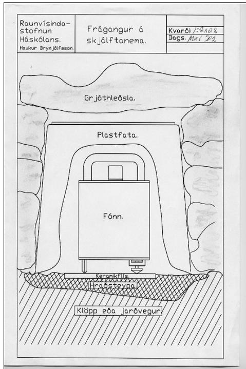
**Figure 6.** A schematic picture of a seismometer installation, drawn by Haukur Brynjólfsson.
