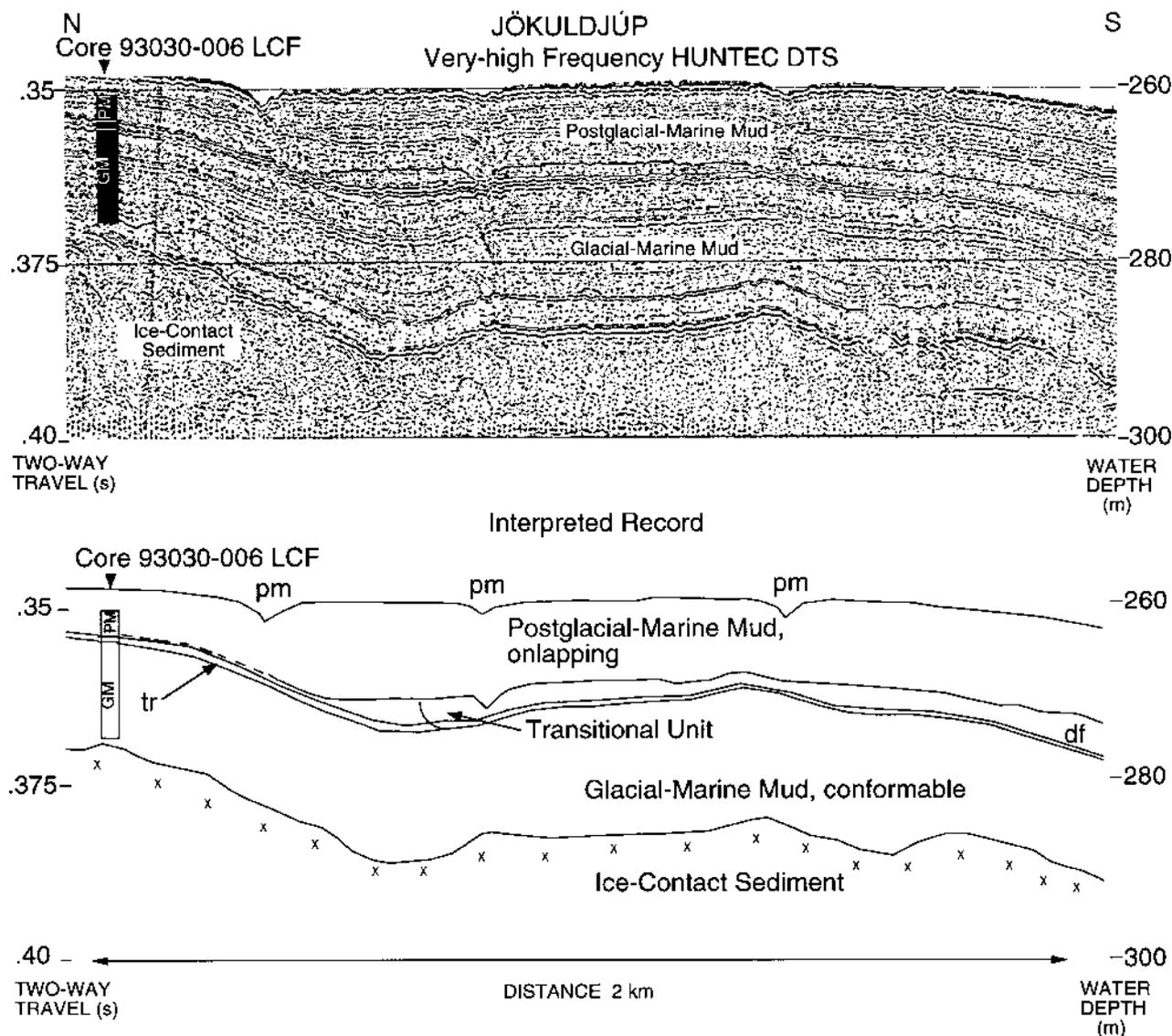
Fig. 3. Hunttec profile (upper) and interpretation of the Hunttec profile (lower) in Jökuldjúp showing placement of 93030-006 LCF within the profile (PM = postglacial marine unit; GM = glacial-marine unit in the core); pm = circular pock marks, 80–100 m in diameter; df = debris flow deposit thickening into deeper water; tr = transitional reflector weakening into deeper water and marked by 30% sand content.
